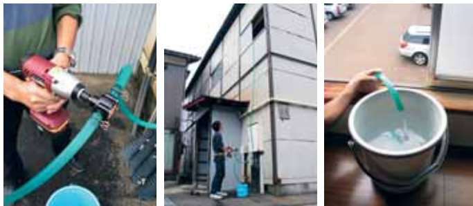
Attached to hand drill Easily lifts water to 2nd floor
