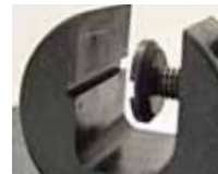
Clamp with grooves to hold calipers securely
