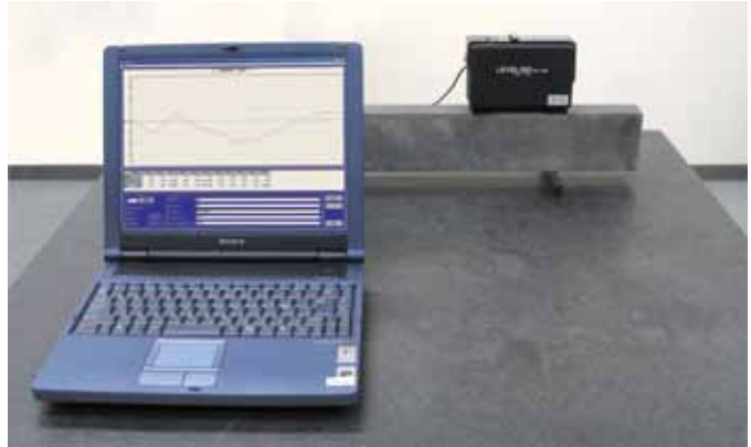
Straightness measurement while connected to PC
