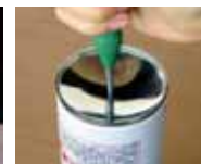
Piercing empty spray can for safe disposal
