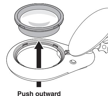
② Insert the new 2x System Lens into the lens frame of the magnifier. ①
