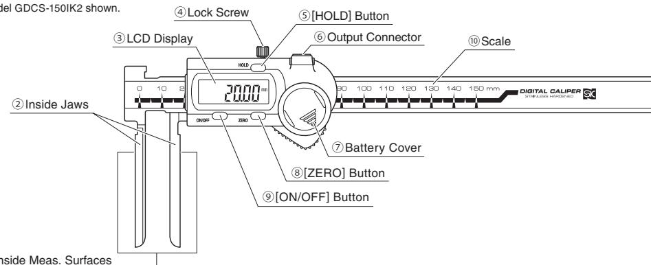
① Inside Meas. Surfaces … Position surfaces inside object to be measured.
